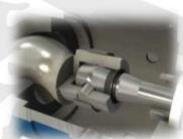
Cross Section of Pin Joint in the Rotor Head
